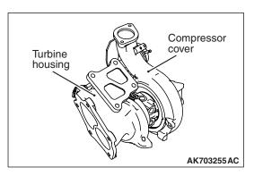
M2150009000286 The turbocharger uses TD05H-152G6-12T: Inconel turbine wheel/ aluminum alloy compressor wheel.
