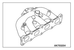
The exhaust manifold made of stainless cast iron is used.
