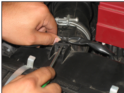
c) Using a small screwdriver disconnect the tree mount zip ties from the stock housing, there are two.
