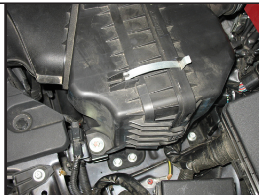
c) Using a small screwdriver disconnect the tree mount zip ties from the stock housing, there are two.
