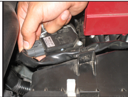
b) Disconnect the mass air flow (MAF) sensor harness from the MAF sensor.
