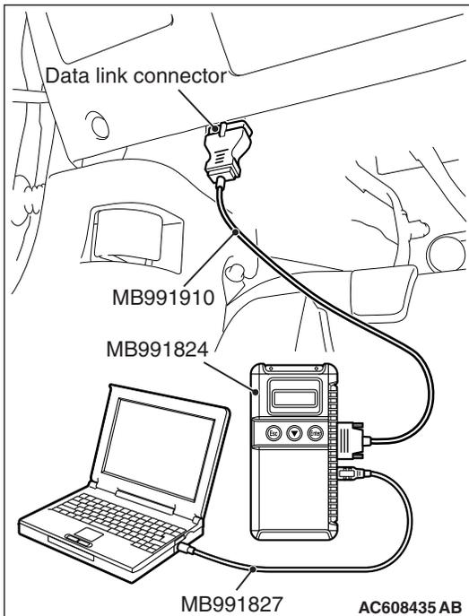
**STEP 2. Using scan tool MB991958, read the engine control module diagnostic trouble code.**
