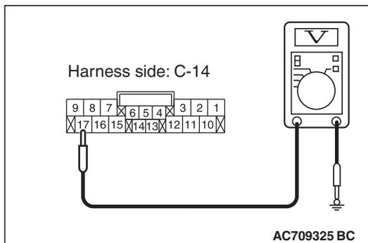
**STEP 6. Check the wiring harness between ETACS-ECU connector C-317 (terminal 1) and multivision display connector C-14 (terminal 17).**
