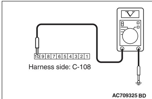
**STEP 8. Check the battery power supply circuit to the CAN box unit. Measure the voltage at CAN box unit connectors C-108.**
