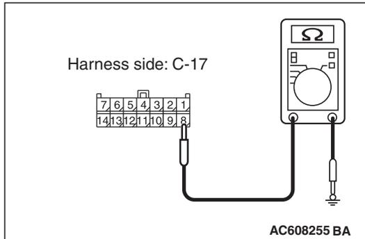
**STEP 2. Check the ground circuit to the satellite radio tuner. Measure the resistance at satellite radio tuner connectors C-17.**
