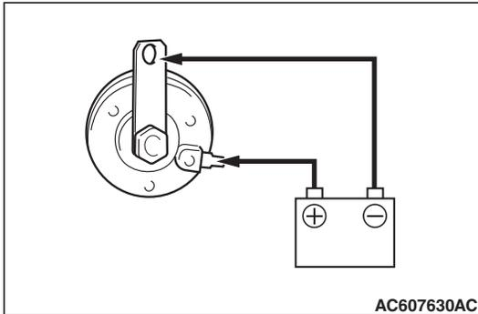
**STEP 10. Check the horn (HIGH) work normally.**
