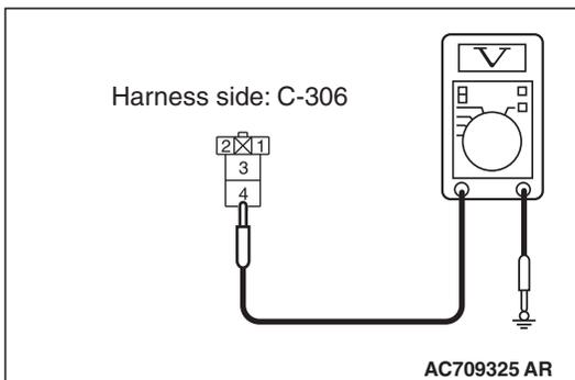
**STEP 11. Measure the voltage at rear window defogger relay connector C-306.**
