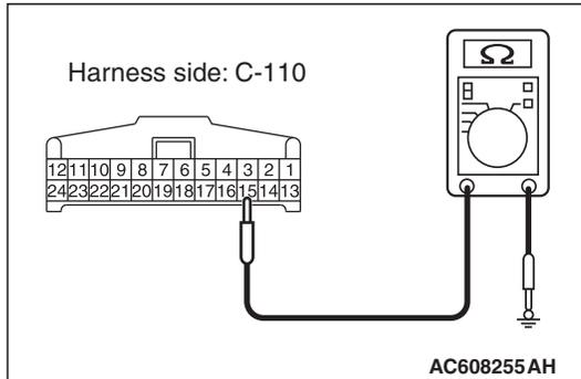
**STEP 2. Check the ground circuit to the hands-free module. Measure the resistance at hands free module connector C-110.**
