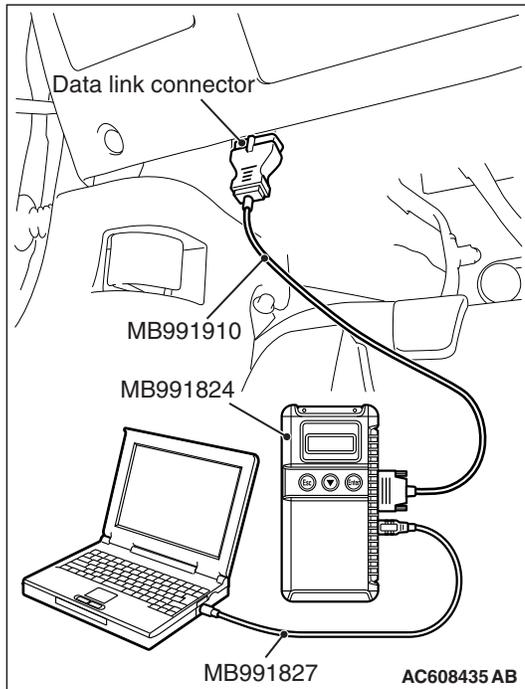
**STEP 2. Using scan tool MB991958, read the satellite radio tuner diagnostic trouble code.**
