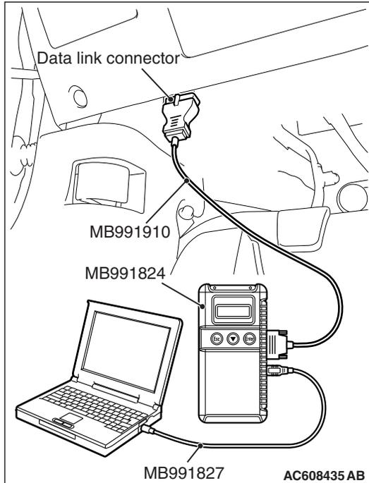
**STEP 2. Using scan tool MB991958, read the SRS-ECU diagnostic trouble code**
