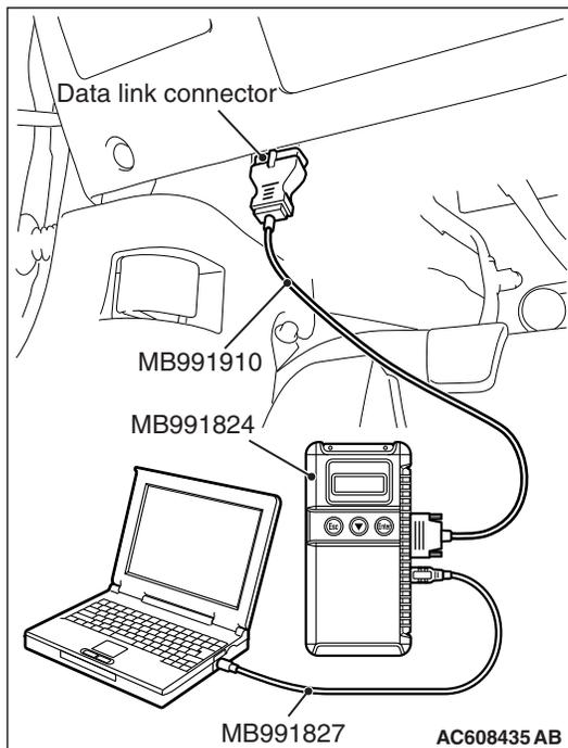
**STEP 2. Using scan tool MB991958 read the combination meter diagnostic trouble code.**
