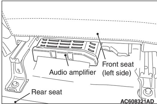
The 8-ch high-power audio amplifier with integrated digital signal processor (total maximum output of 710 W) equipped with the front seat (left side) has been combined with the 9-speaker 7-position system, adopting the Rockford Fosgate® premium sound system. The audio amplifier offers the clear treble without distortion.
