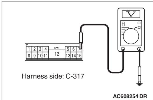
**STEP 2. Check the ignition switch (ACC) line of the power supply circuit to the ETACS-ECU. Measure the voltage at ETACS-ECU connector C-317.**
