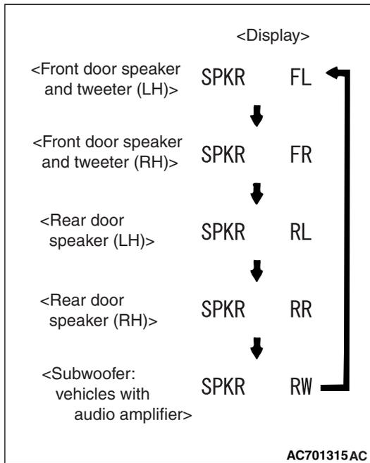
3. Check that the speaker, which is displayed on the center panel display, sounds (If the [CH6] button is pressed, the speaker will be changed).
