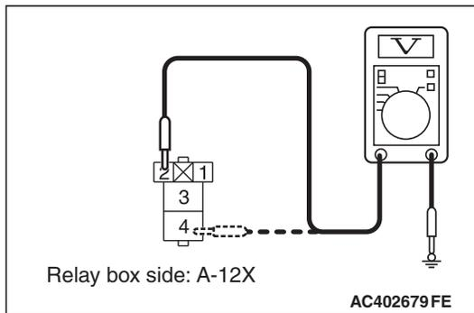
**STEP 4. Measure the voltage at horn relay A-12X.**
