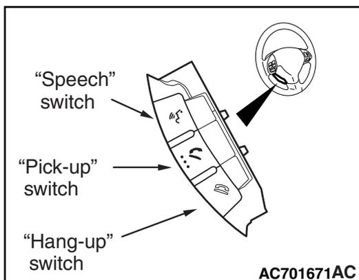
The 4-digit passcode set by security function can be erased by operating the hang-up switch.
