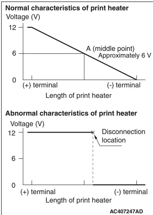
1. Let the engine run (2,000 r/min), and check the printed heater with the battery fully charged.
