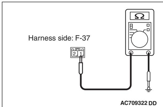
**STEP 5. Check the wiring harness between liftgate switch connector F-37 (terminal 1) and ground.**
