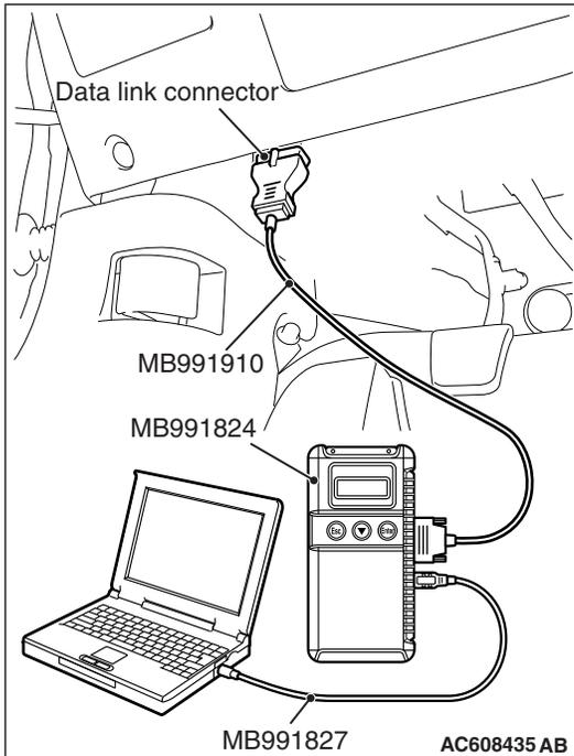
**STEP 3. Using scan tool MB991958, diagnose the CAN bus line.**
