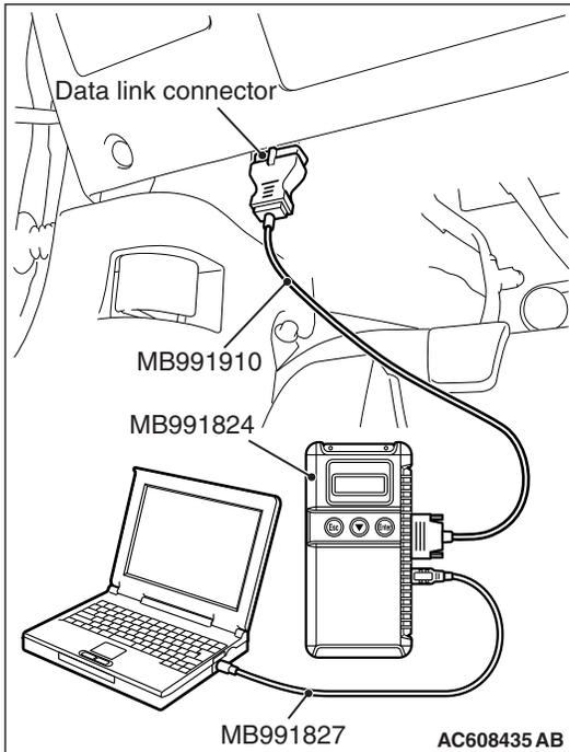
**STEP 3. Check keyless operation system <KOS> or keyless entry system <WCM>.**
