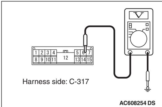
**STEP 3. Check the ignition switch.**
