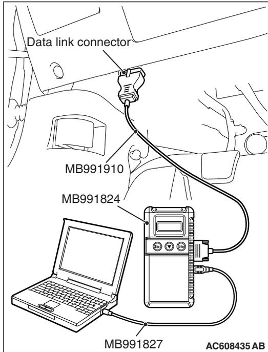
**STEP 4. Using scan tool MB991958 read the radio and CD player <vehicles without MMCS> or CAN box unit <vehicles with MMCS> diagnostic trouble code.**
