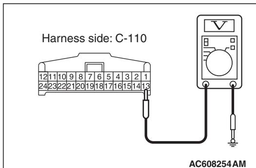
**STEP 4. Check the power supply circuit to the hands-free module. Measure the voltage at hands-free module connector C-110.**
