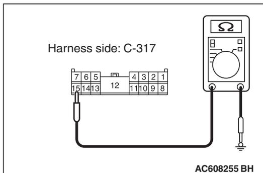
**Q: Is the measured resistance 2 ohms or less?**
