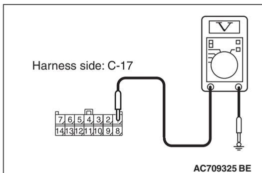
**STEP 5. Check the wiring harness between satellite radio tuner connector C-17 (terminal 1) and fusible link (36).**
