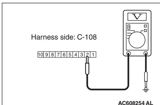
**STEP 5. Check the wiring harness between CAN box unit connector C-108 (terminal 2) and fusible link (36).**
