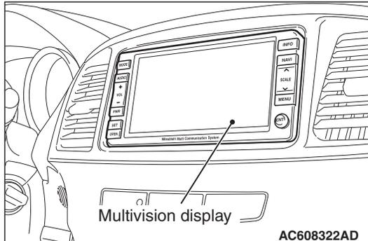
To the Mitsubishi multi-communication system (MMCS), the multivision display (7-inch liquid crystal display of wide 2 DIN size) with built-in hard disk drive (40 GB) and CD/DVD drive has been installed. (The map data includes Hawaii, Alaska, Puerto Rico, and the Virgin Islands.)
