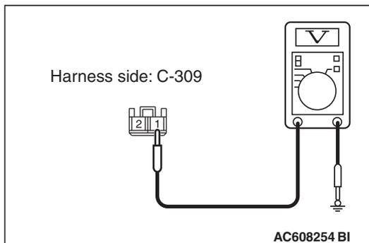
**Q: Is the measured voltage approximately 12 volts (battery positive voltage)?**
