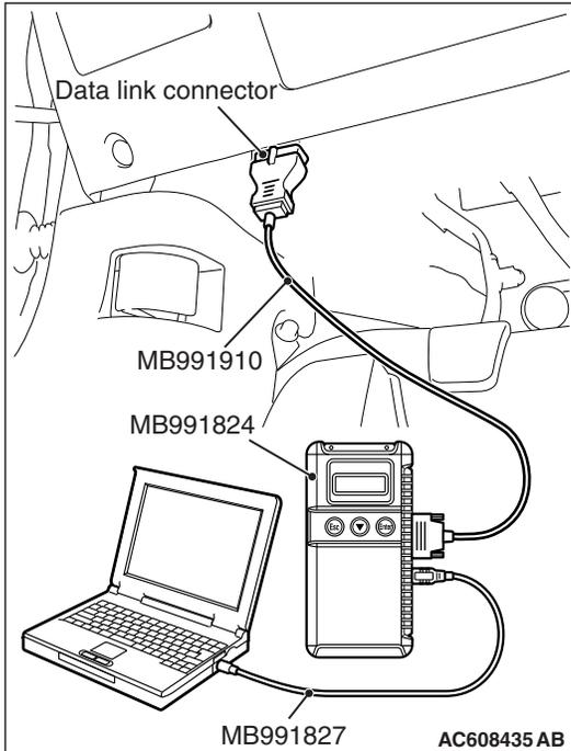
**STEP 2. Using scan tool MB991958, read the hands free module diagnostic trouble code.**
