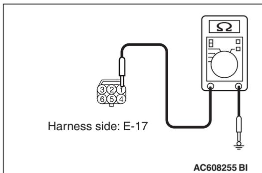
**STEP 5. Check the wiring harness between front door lock actuator (LH) connector E-17 (terminal 1) and ground.**
