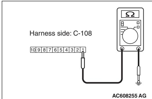
**STEP 2. Check the ground circuit to the CAN box unit. Measure the resistance at CAN box unit connector C-108.**
