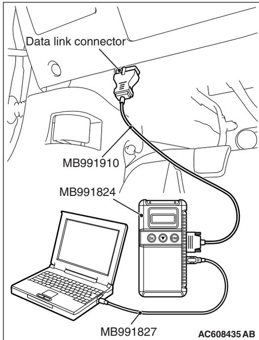
**STEP 1. Using scan tool MB991958, check data list.**
