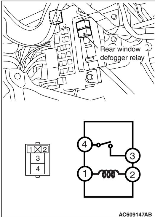
**STEP 7. Check the rear window defogger relay continuity.**
