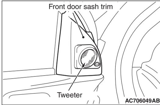
For the front door sash trim, two types of tweeters, the balanced dome tweeter <Vehicles with 6 speakers> and soft dome tweeter <Vehicles with 9 speakers 7 position system>, have been established. The soft dome tweeter can play clearer treble with less distortion compared to the balanced dome tweeter.
