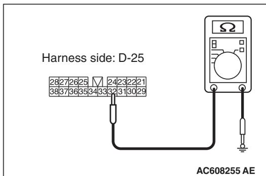
**STEP 14. Check the ground circuit to the rear monitor.
