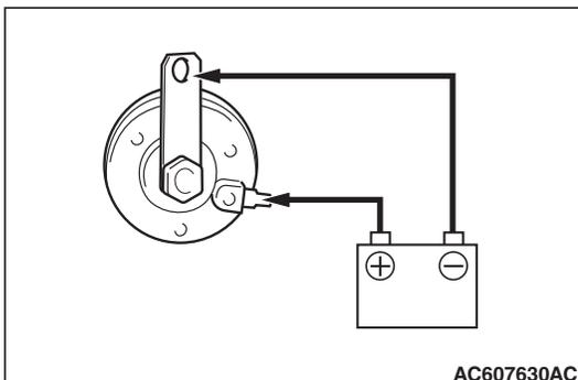
**STEP 13. Check the horn (LOW) work normally.**
