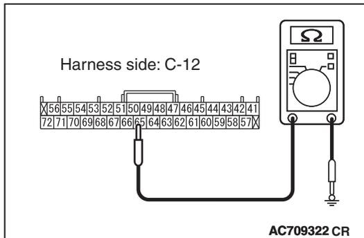
**STEP 2. Check the ground circuit to the multivision display connector. Measure the resistance at multivision display connector C-12, C-14.**
