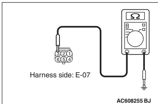
**STEP 11. Check the wiring harness between front door lock actuator (RH) connector E-07 (terminal 3) and ground.**
