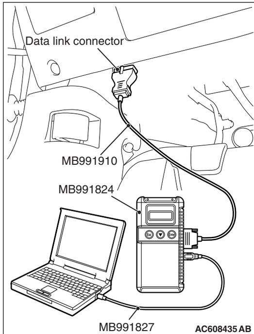
**STEP 2. Using scan tool MB991958, read the occupant classification-ECU diagnostic trouble code.**
