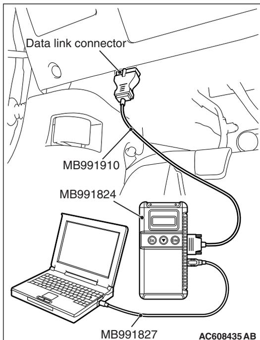
**STEP 2. Check whether the scan tool MB991958 can communicate with the satellite radio tuner.**
