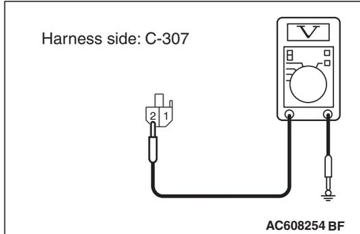
**STEP 6. Check the battery power supply circuit to the ETACS-ECU. Measure the voltage at ETACS-ECU connector C-307.**
