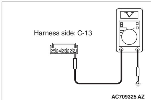
**STEP 9. Check the wiring harness between ETACS-ECU connector C-317 (terminal 1) and multivision display connector C-13 (terminal 21).**
