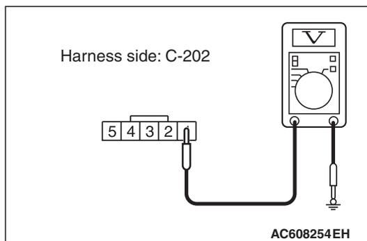
**STEP 3. Check the wiring harness between steering wheel audio remote control switch connector C-202 (terminal 5) and ground.**
