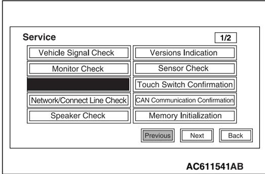
2. The sensor check with the vehicle stationary will be executed in accordance with the screen.
