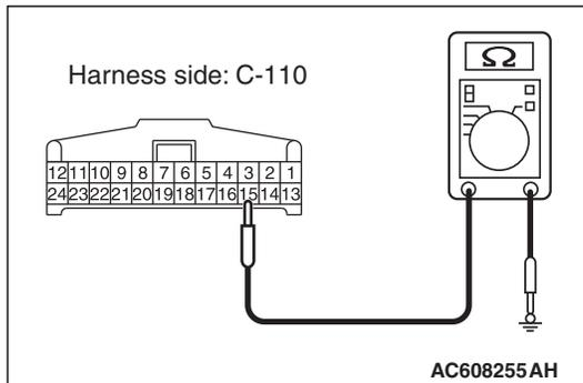
**STEP 5. Check the ground circuit to the hands free module. Measure the resistance at hands free module connector C-110.**
