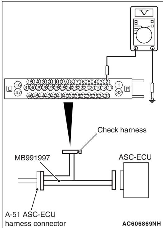
**STEP 14. Voltage measurement at the A-51 ASC-ECU connector**
