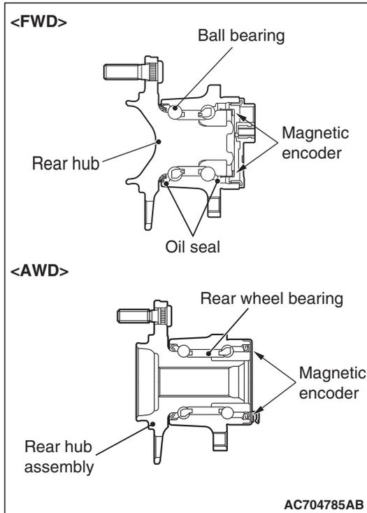
**STEP 7. Check of wheel speed detection encoder**
