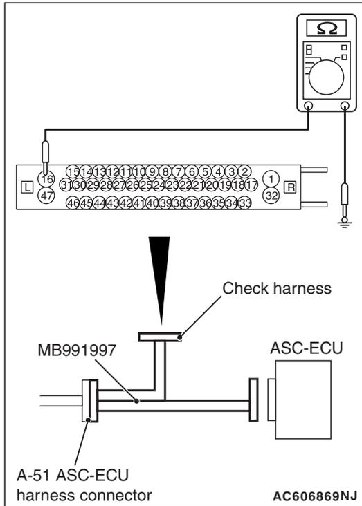
**STEP 18. Resistance measurement at the A-51 ASC-ECU connector**
