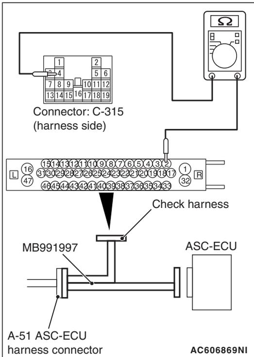
**STEP 17. Resistance measurement at A-51 ASC-ECU connector**
