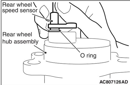
1. Align the mounting bolt hole position of rear wheel speed sensor with the mounting bolt hole position of rear wheel hub assembly.
