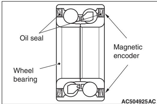
**STEP 7. Check of wheel speed detection encoder**
