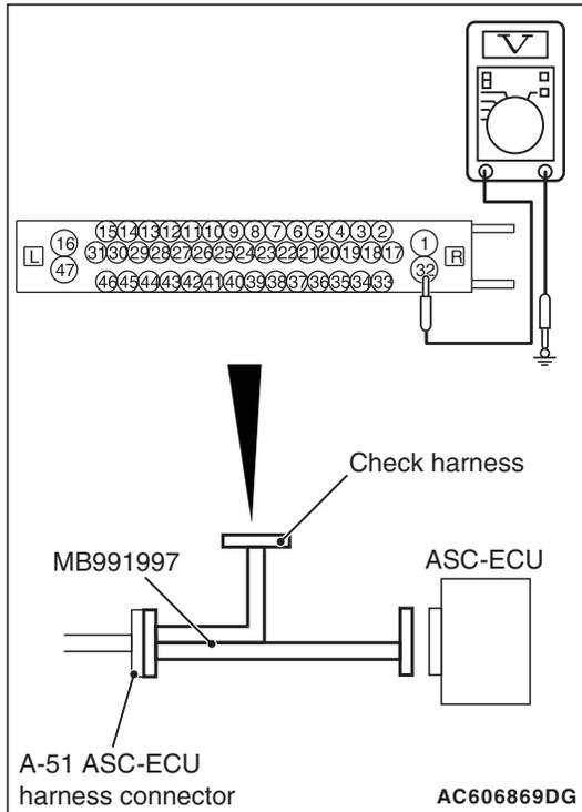
**STEP 8. Voltage measurement at the A-51 ASC-ECU connector**
