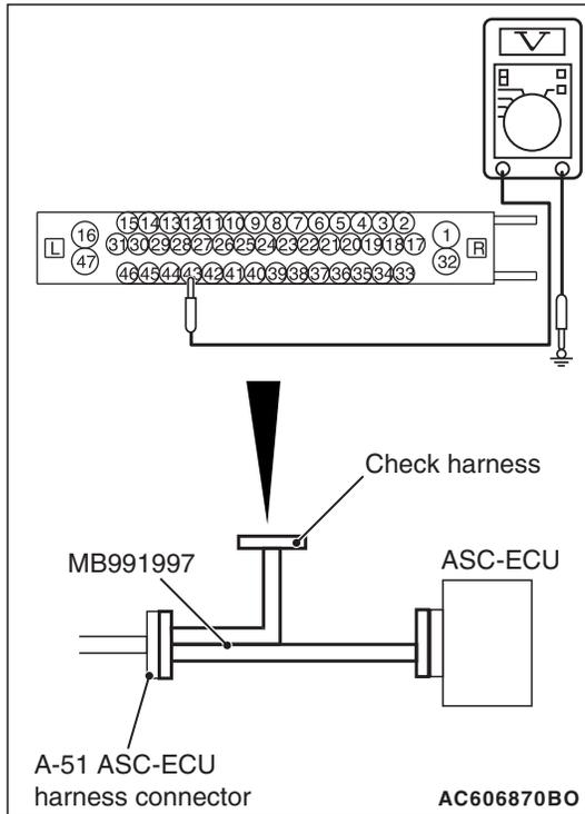
**STEP 7. Voltage measurement at the A-51 ASC-ECU connector**
