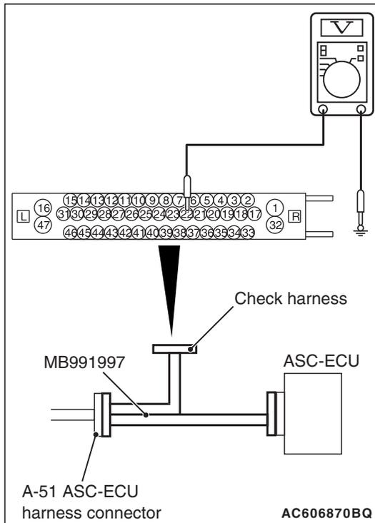
**STEP 9. Voltage measurement at A-51 ASC-ECU connector**
