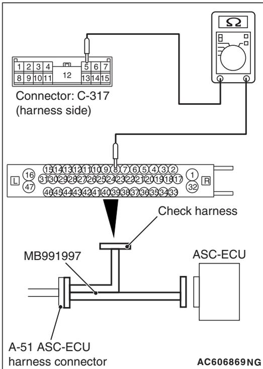
**STEP 13. Resistance measurement at A-51 ASC-ECU connector**
