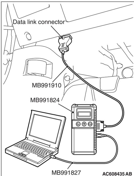
**HOW TO PERFORM ACTUATOR TEST****Required Special Tools:**
