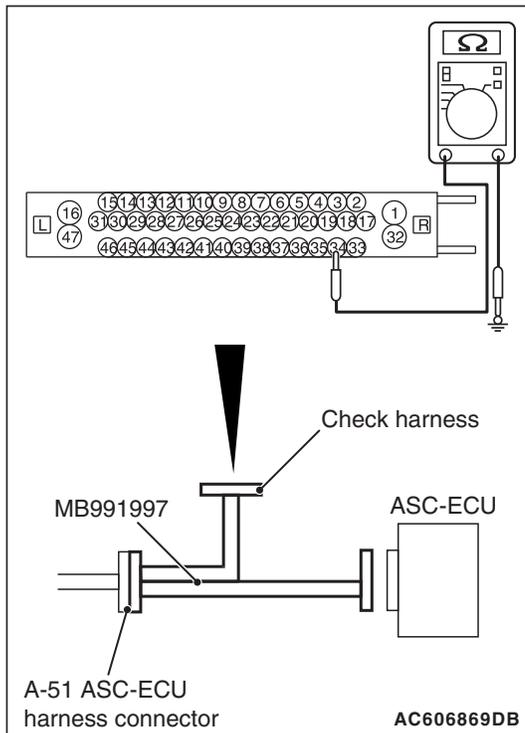
**STEP 7. Resistance measurement at A-51 ASC-ECU connector**
