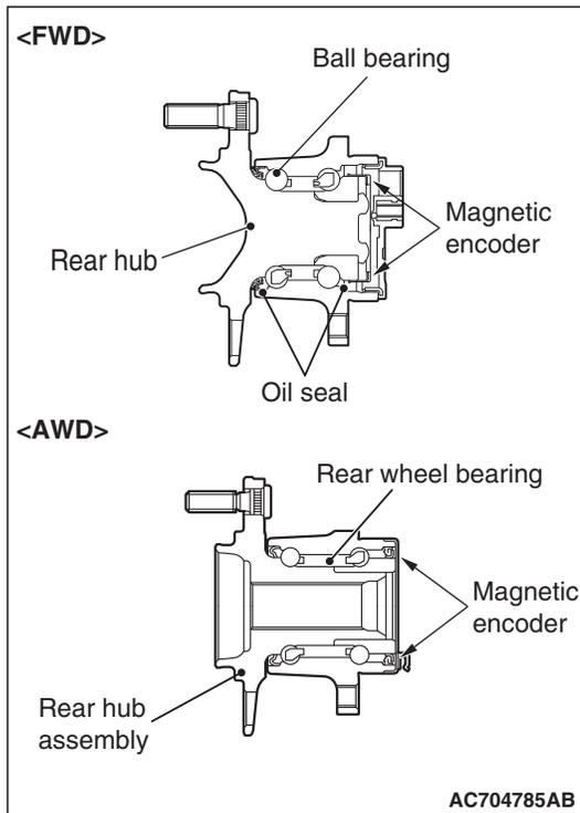
**STEP 4. Check of wheel speed detection encoder**
