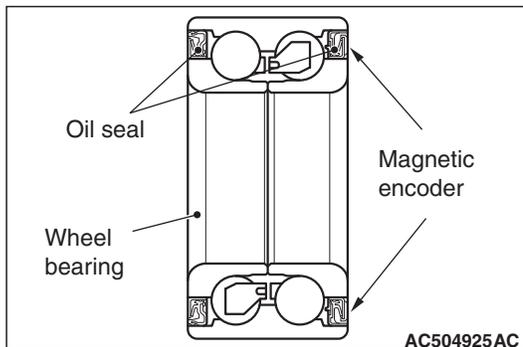
**STEP 13. Check of wheel speed detection encoder**
