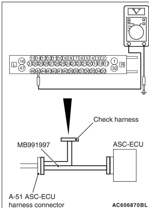
**STEP 13. Connector check: A-51 ASC-ECU connector, A-07 wheel speed sensor <FL> connector**
