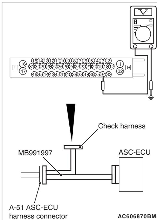
**STEP 13. Connector check: A-51 ASC-ECU connector, A-02 wheel speed sensor <FR> connector**
