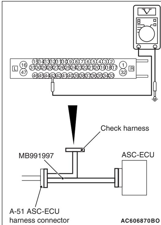
**STEP 12. Voltage measurement at the A-51 ASC-ECU connector**
