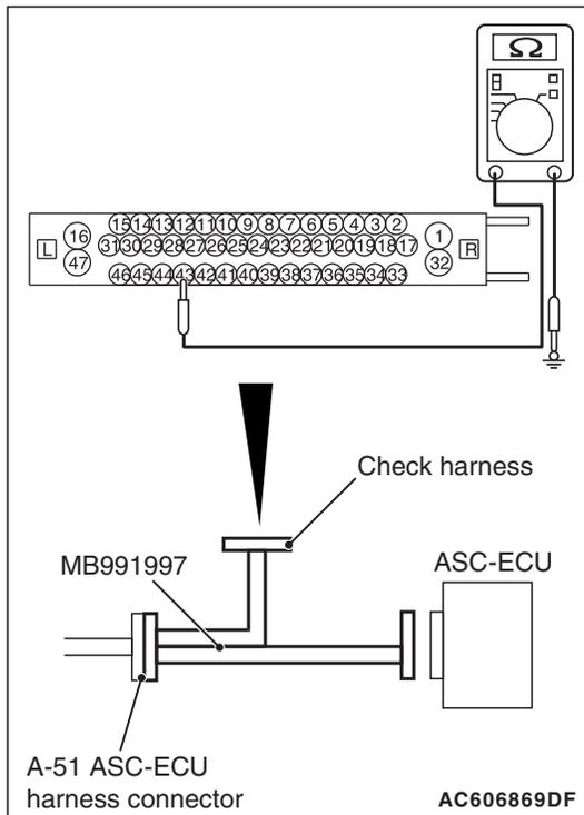
**STEP 6. Resistance measurement at A-51 ASC-ECU connector**
