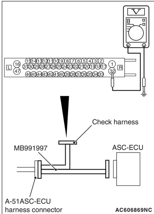
**STEP 4. Voltage measurement at the A-51 ASC-ECU connector**
