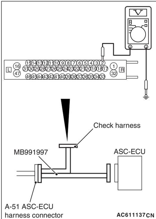
**STEP 5. Voltage measurement at the A-51 ASC-ECU connector**
