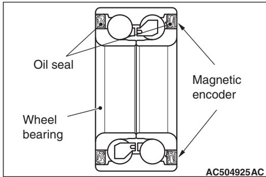
**STEP 4. Check of wheel speed detection encoder**
