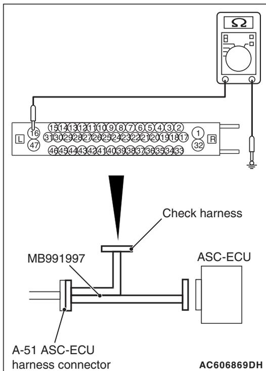
**STEP 9. Resistance measurement at A-51 ASC-ECU connector**
