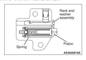
The tensioner maintains the tension of the timing chain. It contains a piston with a built-in spring. With the tensioner installed, its piston directly pushes on the tension lever in order to automatically adjust the tension of the timing chain.
