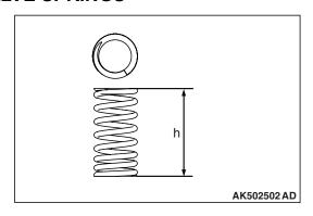
To prevent the engine from surging at high speeds, unequal-pitch springs are used.
