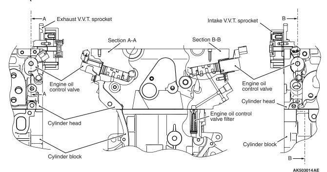
The MIVEC consists of the parts shown in the illustration.
