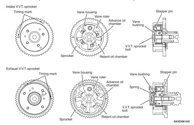
The engine oil control valve controls the hydraulic pressure in order to move the vane rotor in the V.V.T.
