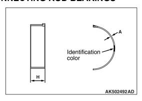
The upper and lower connecting rod bearings are the same. Each connecting rod bearing is provided with a backing plate. Its bearing portion is made of an aluminum alloy and its backing plate is made of ordinary sheet steel.
