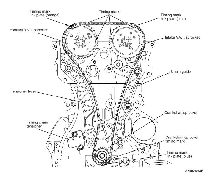
The two camshafts are driven by the timing chain via the camshaft sprockets.
