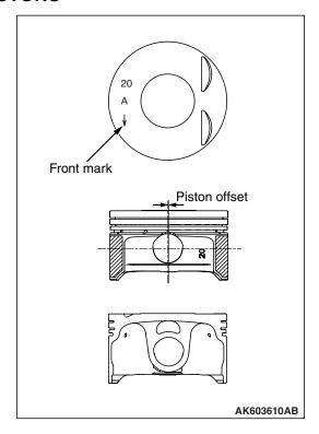
The pistons are made of a special aluminum alloy. Their weight has been reduced by lowering their overall height and increasing the depression at each end of the piston pin.
