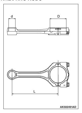
The connecting rods are made of highly rigid, forged carbon steel. The cross section of the rod portion is shaped like the letter H.
