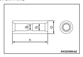
The piston pins are the semi-floating type. Each pin is press-fit and secured in the small end of the connecting rod, while it floats in the piston.
