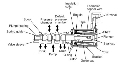
The engine oil control valve consists of a solenoid valve, which switches the hydraulic pressure that acts on the vane rotor in the V.V.T. sprocket assembly. This valve is actuated by a signal from the engine ECU.
