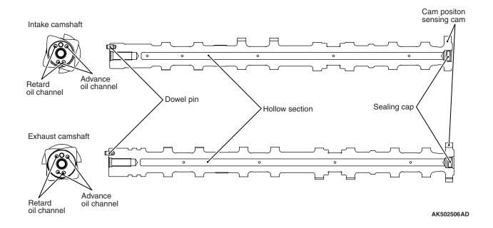
The camshaft are hollow for weight reduction. Each camshaft is provided with an oil passage to guide the hydraulic pressure from the engine oil control valve to the V.V.T. sprocket.
