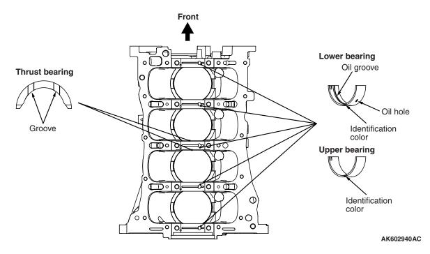
The upper crankshaft bearings have oil grooves and the lower crankshaft bearings do not.
