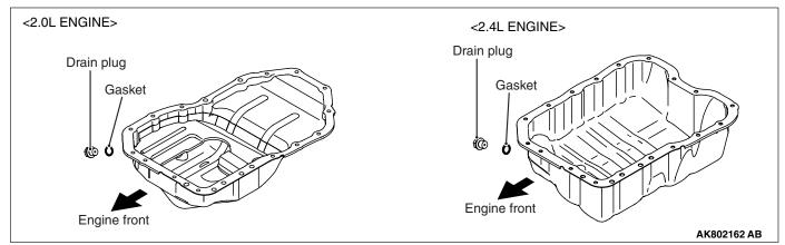
The oil pan is made of high damping sheet metal and contains an oil sump in the forward area of the engine.
