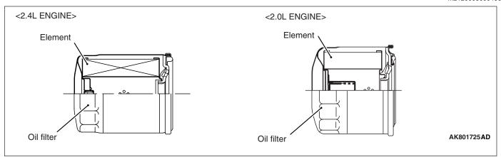
The oil filter is installed to the bracket placed at the left side of ladder frame.
