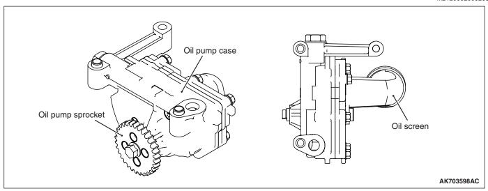
The oil screen is integrated into the oil pump case to be compact and lightweight.
